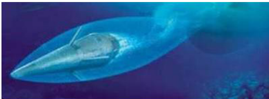
Figure 5: “Super Cavitating” Torpedo - Shkval
